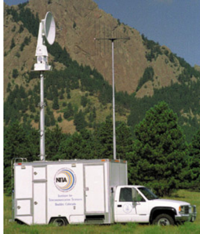
Figure 6 – NTIA mobile Radio Spectrum Measurement System (RSMS)
