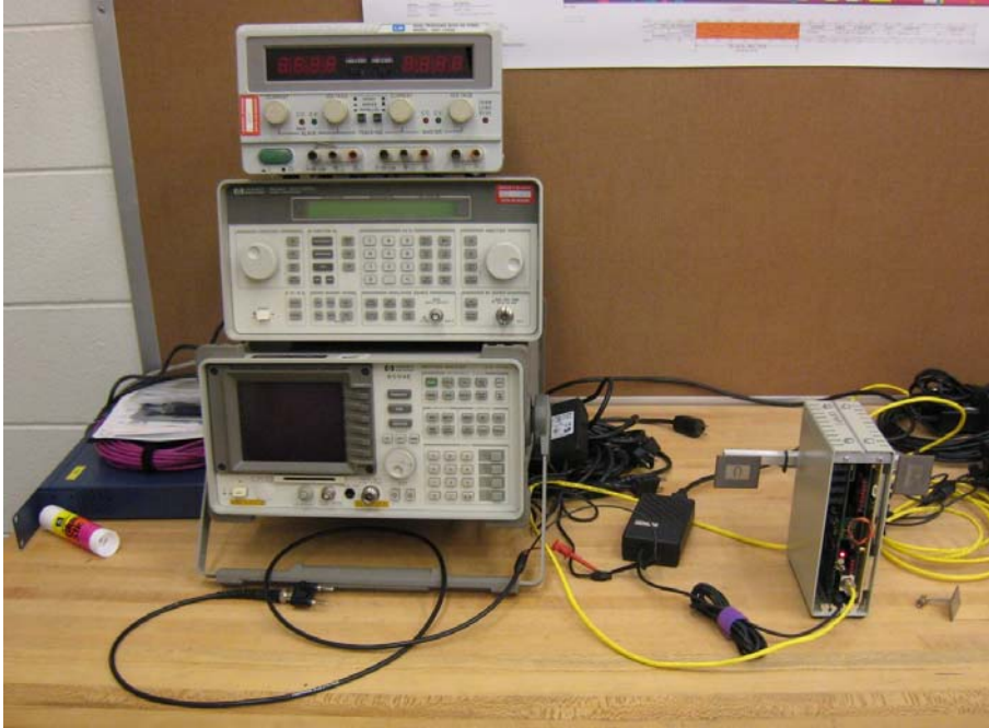
Figure 46 – HP spectrum analyzer and KUAR calibration setup
